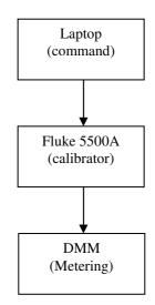
Figure 1. Block diagram of the calibration system
