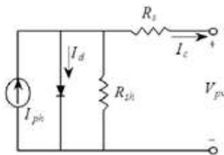
Figure 2. Model of photovoltaic using single battery
