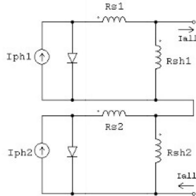
Figure 3. Model of PV circuit array
