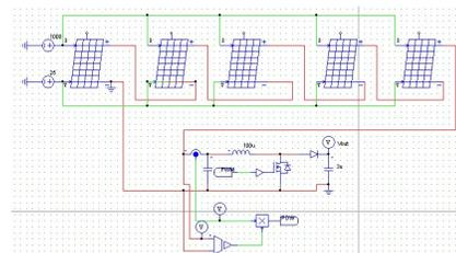
Figure 4. Model of PV on PSIM
