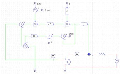
Figure 6. Equivalent circuit of battery circuit modeling
