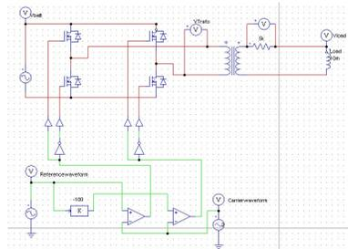
Figure 7. Single Phase Inverter Circuit
